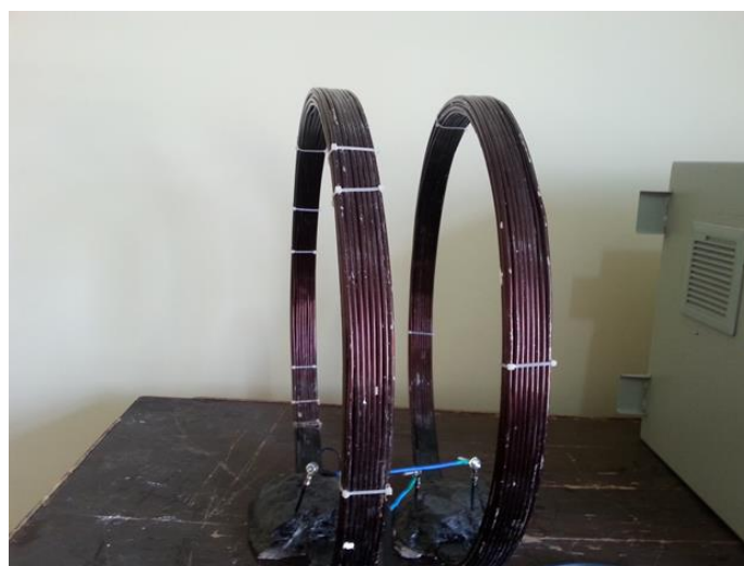
Figure 1. Helmholtz coil used in this study to expose the rats to the 50 Hz, 1 mT MF
