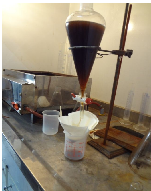
Figure 1. Separating the alkali phase from the aqueous phase of the base hashish solution after adding chloroform and isopropanol by decanting and using filter paper.
