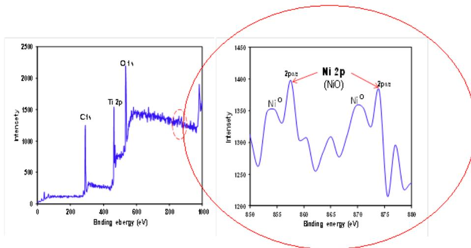
**Figure 4.** XPS spectrum of Ni 2p peaks and satellites for TiO<sub>2</sub> particles after reduction process.
