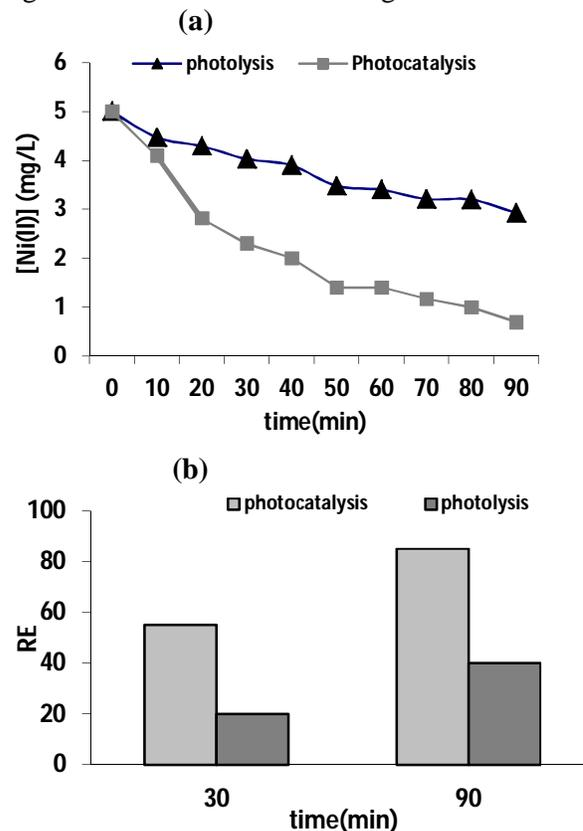
**Figure 3.** The variation of Ni(II) concentration versus time (a), and comparison of *RE* values after two different times (b) for the photolysis and photocatalysis processes; pH = 9.2, [TiO<sub>2</sub>] = 42 mg/L, and *T* = 34 °C.
