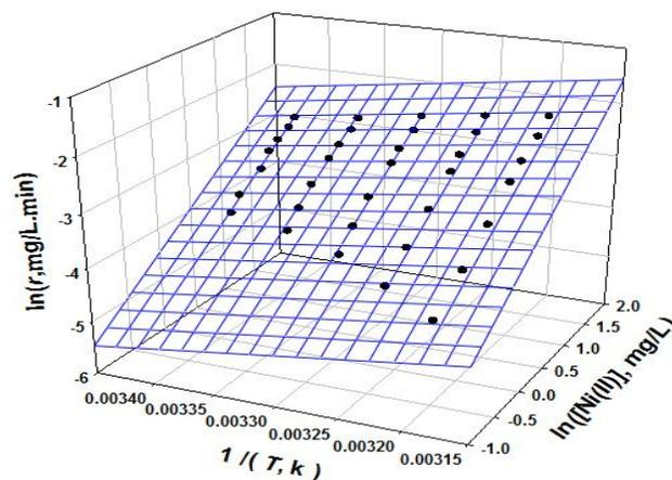
**Figure 5.** Correlation diagram for experimental kinetic data, pH of 9.2, and [TiO<sub>2</sub>] = 42 mg/L.
