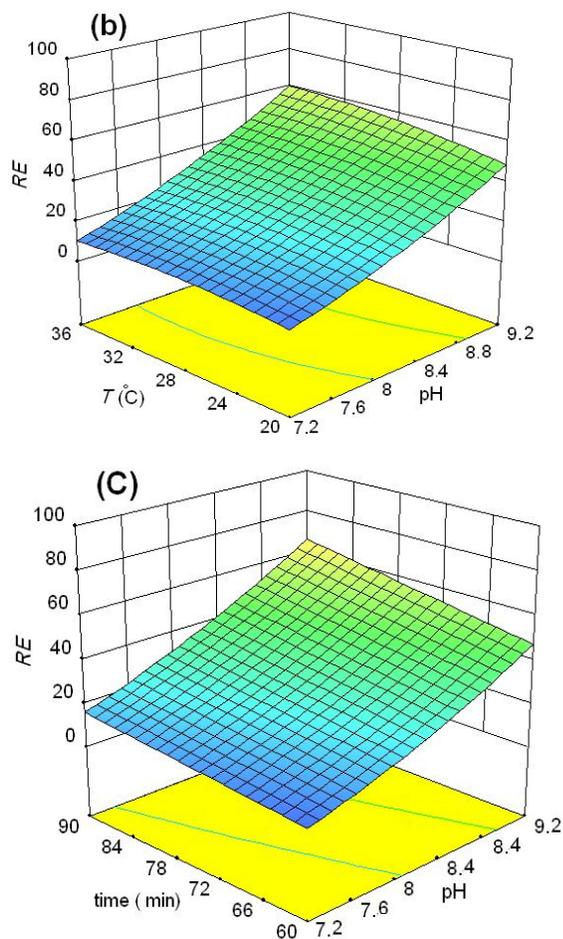
**Figure 2.** The response surface plots showing the effect of: (a) TiO<sub>2</sub> particles dosage and solution pH at temperature of 28 °C and reaction time of 75 min (central point), (b) temperature and pH with TiO<sub>2</sub> particles dosage of 25 mg/L and reaction time of 75 min, (c) reaction time and pH at temperature of 28 °C and TiO<sub>2</sub> dosage of 25 mg/L.
