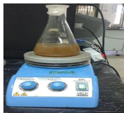
Figure 2. \text{Fe}/\text{S}_2\text{O}_8^{2-} process reactor.
