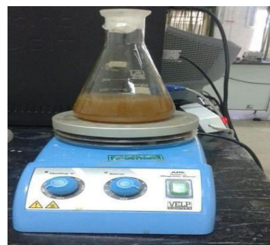
Figure 2. \text{Fe}/\text{S}_2\text{O}_8^{2-} process reactor.
