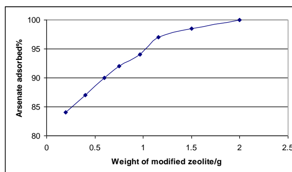
Figure 6 Arsenate anion removal by modified natrolite zeolite in different quantities
