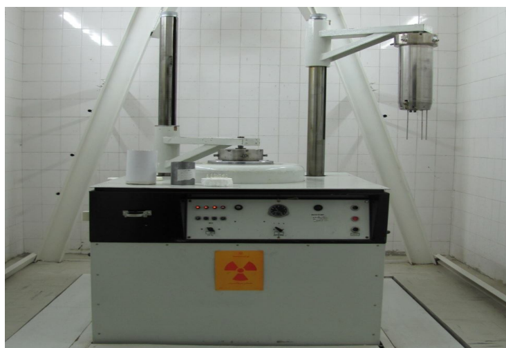
Figure 1. Gamma cell device, model PX-30, Nuclear Energy Organization, Beam Application Research Institute, Tehran, Iran.
