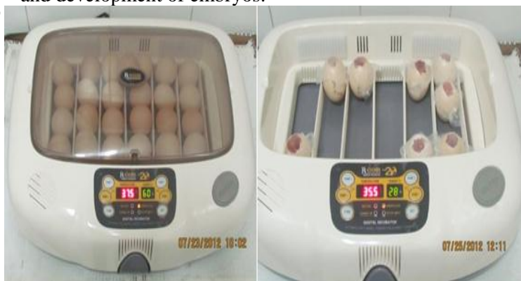
Figure 1. The fertilized eggs were incubated in vertical position at 37°C± 0.5 and 60% humidity.
