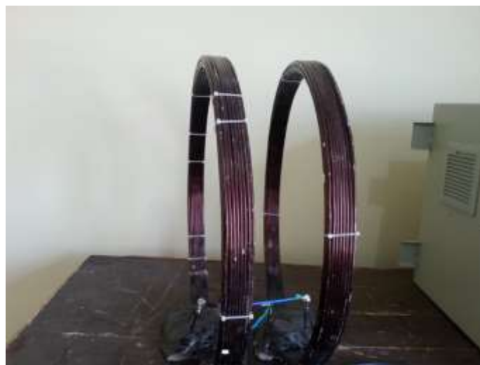
Figure 1. Helmholtz coil used in this study to expose the rats to the 50 Hz, 1 mT MF
