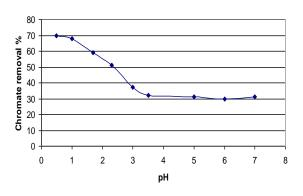
Figure 7 The removal efficiency of chromate ion in different pHs
