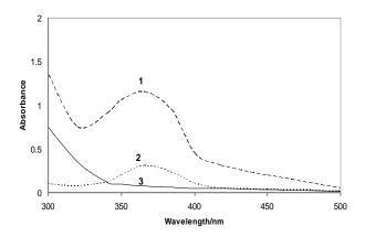
**Figure 9** UV-visible spectrum absorbance of chromate ions with different 0.001 and 0.0001 molar concentrations (before zeolite application) and also, after application of modified zeolite in optimum operating conditions
