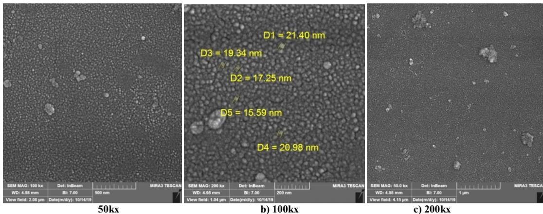
**Figure 3.** Images of colloidal Ag nanoparticles by scanning electron microscopy (SEM).
