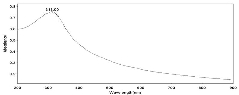
**Figure 2.** UV-visible absorption spectra of the synthesized TiO<sub>2</sub> nanoparticles. The absorption peak was obtained in the visible range at 313nm.
