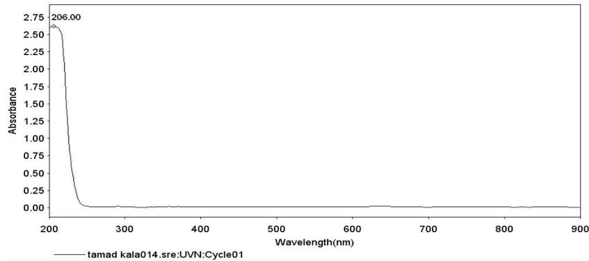
**Figure 1.** UV-visible absorption spectra of synthesized Ag nanoparticles. The absorption peak was obtained in the visible range at 206nm.
