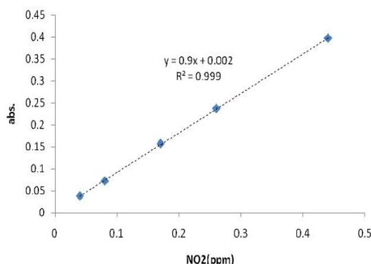
NO<sub>2</sub> calibration curve in density of 0.04 to 0.44 μg.ml in 550 nm wavelength has line equation of A= 0.9C+0.002 and R<sup>2</sup>=0.999.
