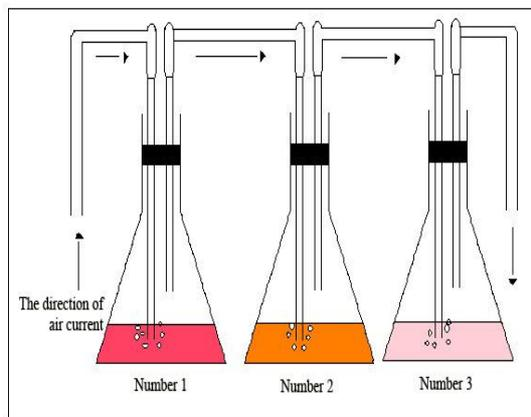
**Figure 1. Absorbing system of NO<sub>x</sub> designed at the library**
